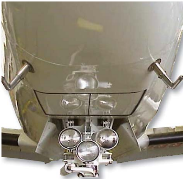
Extended Nose with Doors Closed — EO/IR Camera Stowed
